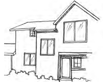
Poor, bland window treatment
