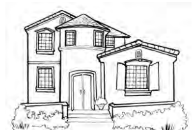
Turret is too large
